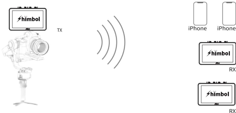
c. One ZO600MS unit under TX mode connects one ZO600MS unit under RX mode and the RX unit of another model of Shimbol brand to work simultaneously.
